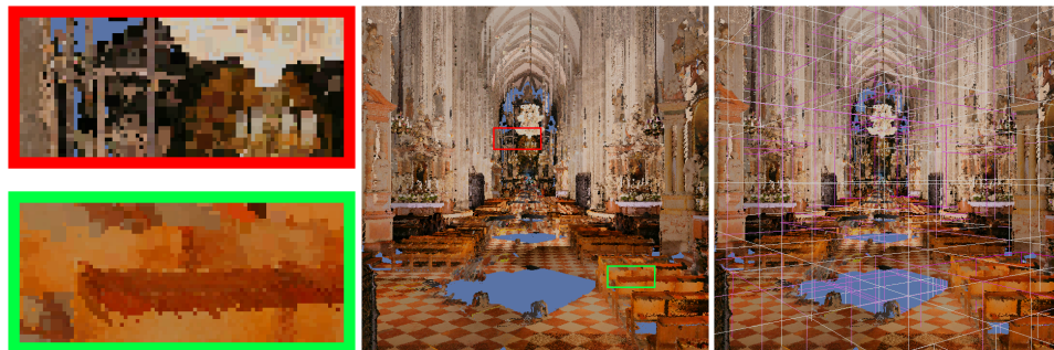
Figure 6.9: Screenshots of the walkthrough in the cathedral model. The zoomed parts of the middle image show that the point sizes are similar for the far away and for the nearby regions, proving that the LOD selection works well. The middle image was rendered with 9,890,458 points in 308 cells, and loading was completed. In the right image, the magenta bounding boxes indicate that some children of these cells were not rendered because the projected sizes of their bounding boxes were too small.
