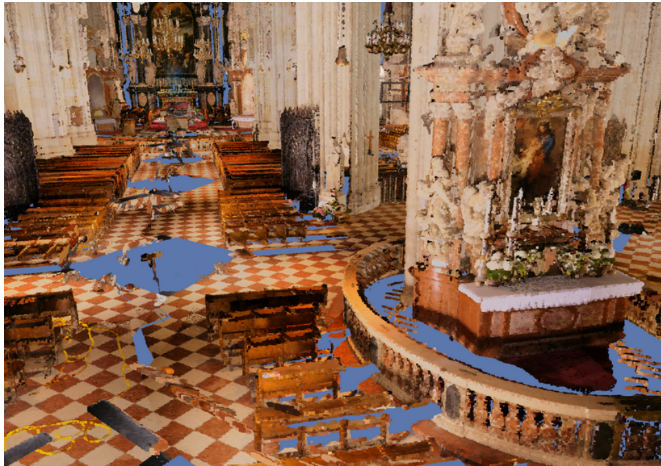
Figure 6.1: Example screenshot of an unprocessed point cloud consisting of 262M points.
